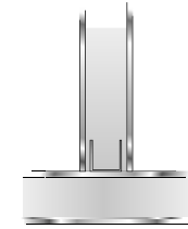
3 Front to partition wall connection
